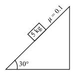
A block of mass 5 kg is placed on a rough inclined surface as shown in the figure. If  $\vec{F_1}$  is the force required to just move the block up the inclined plane and  $\vec{F_2}$  is the force required to just prevent the block from sliding down, then the value of  $\left| \vec{F_1} \right| - \left| \vec{F_2} \right|$  is ; [Use  $g = 10 \text{m/s}^2$ ]
