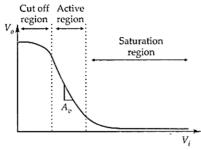
The active region of the transfer characteristic is used for the amplification purpose. This is because in this region,  $I_C$  increases almost linearly with the increase of  $V_i$ .
