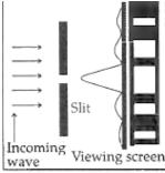
Secondary maxima keep on getting weaker in intensity, with increasing n. This is because, at the
